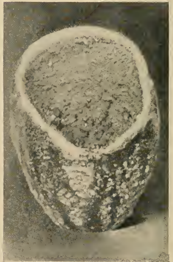
Fig. 39—Crucible squeezed out of shape by tongs
